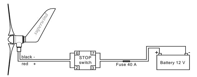
Wiring scheme shows connection without marine charge regulator.
